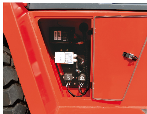
Independent integrated electric cabinet
